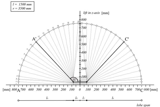
Fig.17: Cross-sectional study measuring folding angle  $\alpha$ .
