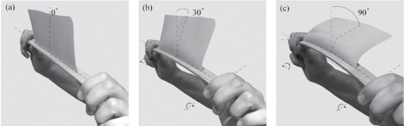
Fig.3: Physical model of the deformation principle of *Strelitzia reginae*. Bending the backbone causes the attached lamina to deflect up to 90° sideways, which is initiated by lateral-torsional buckling.
